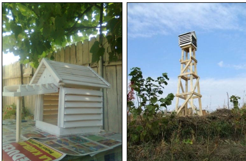
Fig. 4. Mini meteorological shelter (left); Mini-shelter at 2 m standard height at Tudora, Jud. Botoșani observation point (right)
